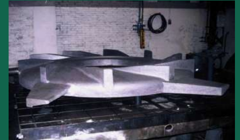
Bladed wheel weight : 4 500 kg GX 5CrNiMoNb 18-12
